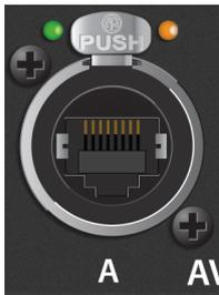
**AVB A.** This locking Ethernet connection should be used to connect your NSB to your AVB network.
