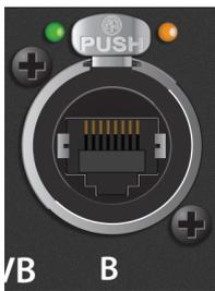
**AVB B.** This locking Ethernet connection can be used to connect your NSB to another NSB or other AVB device. You can also use this connection to daisy chain additional NSB stage boxes or EarMix 16M personal monitor mixers in situations where you are connecting your devices directly to your mixer without an AVB switch or if you have exhausted the available ports on your AVB switch.
