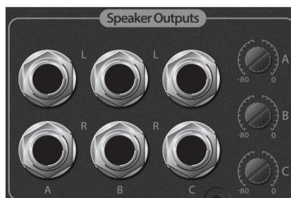
**Speaker A L/R Outputs:** Connect your primary powered- speaker system to the balanced A L/R Speaker Outputs.
