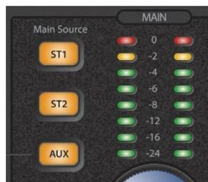
**Main Source Buttons:** The Main Source buttons select the audio for the Speaker Output jacks, the Main L/R Line Outputs, and any headphone amplifiers whose Source switch is set to its Main position (up).
