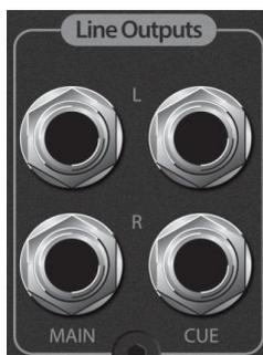
**Main L/R Line Outputs:** Monitor Station V2 passes input audio sources directly to the Main L/R Line Outputs. These outputs derive their signal directly from the currently selected Main input sources and are unaffected by the Main level-control knob and the Mono, Mute, and Dim buttons.
