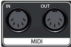
**MIDI I/O.** These are the MIDI input and output connections. MIDI stands for “Musical Instrument Digital Interface.” However, MIDI can be used for many things other than instruments and sequencing. The MIDI inputs and outputs allow connection to a variety of MIDI-equipped hardware, such as keyboard controllers, and can be used to send and receive MIDI Machine Control and MIDI Time Code.
