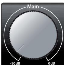
**Main.** The Main knob can control any or all of the outputs on the rear panel of your Quantum and has a range of -80 dB to 0 dB. In addition to level control, the main outputs have the following controls:
