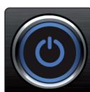
**Power button and Sync light.** The lighted ring around the power button of your Quantum is a clock source / sync indicator. It lets you know if your unit is receiving word clock correctly.
