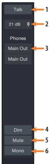
1. **Talk Button (Quantum).** Use this to engage the Talk function. This will route the onboard talkback microphone to the cue mix outputs.
