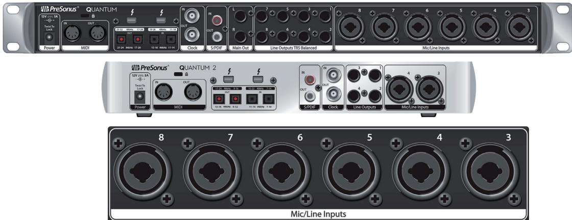
**Rear-panel Mic Inputs.** As previously mentioned in Section 2.1, additional microphone preamps are available on the rear of your Quantum interface.
