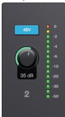
The inputs on your Quantum-series interface are auto-sensing. When an XLR cable is connected, controls for the microphone preamp will be available in UC Surface. These controls include a fully variable gain control and phantom power as well as input metering.
