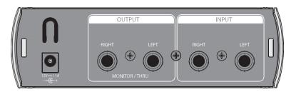
Left/Right Balanced Inputs. These line-level inputs should only be used for signals from sources that do not require preamplification, such as CD and MP3 players, mixers, and audio interfaces. Left/Right Balanced Inputs. 这些线级输入只能用 于不需要前置放大的信号源,如CD和MP3播放器、 混音器和音频接口。
