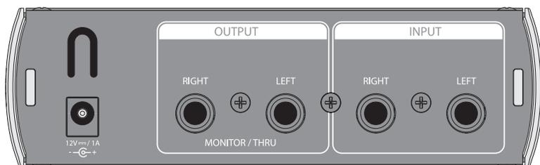
**Left/Right Balanced Inputs.** These line-level inputs should only be used for signals from sources that do not require preamplification, such as CD and MP3 players, mixers, and audio interfaces.
