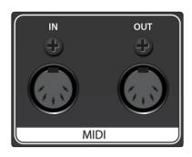
**MIDI I/O.** MIDI stands for "Musical Instrument Digital Interface." MIDI inputs and outputs allow connection to, and communication with, external MIDI equipment. One function of these ports is MIDI sequencing but the MIDI protocol can be used for much more than instruments and sequencing.
