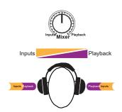
**Power User Tip:** When monitoring your inputs through Studio One or another DAW, it is important that you turn the Mixer knob all the way to the Playback position. Monitoring both the input signal and the playback stream will create a doubling effect that will make monitoring difficult.
