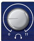
**Phones.** The Phones knob controls the volume of the headphone output on the rear of the unit. The headphone amplifier is quite powerful, and the volume goes to 11, so use the maximum setting with extreme caution.
