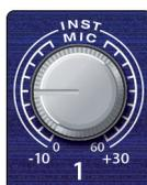
**Input Gain/Trim Control.** These knobs provide the following gain structure:
