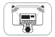
The speakers should be separated so that the tweeters form an equilateral triangle with your head. The monitors should be "toed in," or angled, so that they are pointed at you, not pointed straight ahead.
