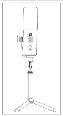
Secure the half-yoke bottom to the threads at the top of the PTS-1 (or other) mic stand.
