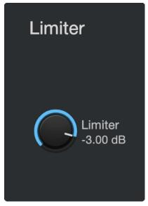
This encoder sets the threshold of the limiter for the selected channel or output bus. When the signal's amplitude (level) exceeds the threshold setting, the limiter is engaged. Turning the knob counterclockwise lowers the threshold, so limiting begins at a lower amplitude. The Limiter ratio is  $\infty$ :1.
