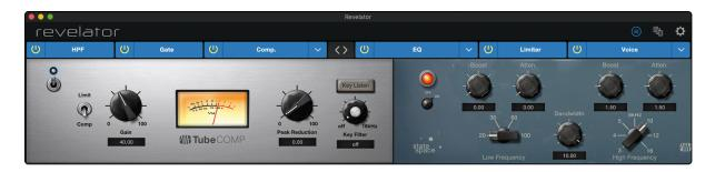
The Fat Channel provides essential vocal processing tools to sculpt your sound, as well as Voice FX section to warp, distort, and bounce it around. These are the effects that are stored with a preset. A dedicated Reverb processor is also available, but it is important to note that Reverb is not stored with a Preset. More on Reverb in the *Fat Channel and Voice Effects section*.
