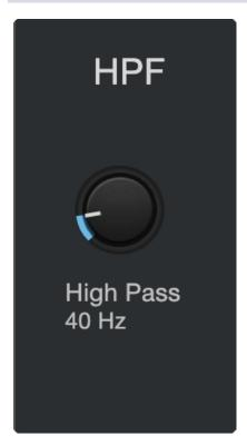
Use this control to set the High-Pass Filter frequency threshold for the selected Channel or Output Bus. The filter's threshold can be set from 24 Hz to 1 kHz. When the threshold is set to its lowest point, the filter is off. The high-pass filter's slope is -12 dB/8va.
