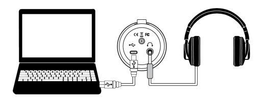
All the connections you need for your Revelator Dynamic are located on the bottom of the microphone.
