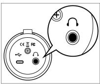
**Headphone Output.** This is the headphone connection for your Revelator Dynamic. The level is controlled by the Volume knob. You can also change the mix that you are listening to from Universal Control. See *the Mixing and Loopback Audio section* for details.
