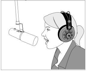
The front of the Revelator Dynamic should always be directed toward the sound source. Use the supplied mount to attach your Revelator Dynamic to a mic stand. A windscreen is integrated into the design of the Revelator Dynamic, so no additional pop filter is needed.
