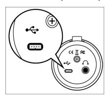
**USB-C® Compatible Connection.** Use this port to connect your Revelator Dynamic to your computer. While the Revelator Dynamic's onboard connection is USB Type C, it is fully compatible with USB Type A 2.0 and 3.0 connections. Use the USB-C to A cable that came with your Revelator Dynamic if your computer has a USB-A connection rather than a USB-C connection. Please note: *Revelator Dynamic is backward compatible with USB 2.0 and USB 3.0 speed connections. USB 1.1 is not supported.*
