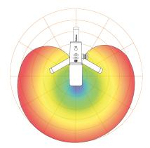
When looking at the shape of this polar pattern, it quickly becomes apparent why holding a microphone too close to the capsule will create problematic handling noise. While this is fine for a stage performance where the sheer volume of the instruments on stage will mask this noise, in an audio recording made from a quiet location, handling noise becomes a distraction from the primary sound source. And in this case, that source is you.
