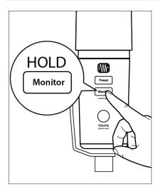
To set your Revelator Dynamic's input level, press and hold the Monitor button. The Volume knob will turn green, letting you know that it is now controlling the microphone level.
