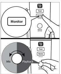
Revelator Dynamic provides an easy way to create a blend between your microphone signal and the playback from your computer. This lets you listen to your performance in real-time without any latency (delay).
