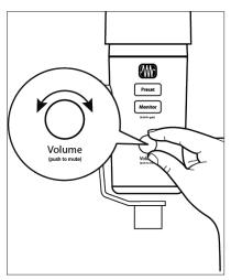
Turn the Volume knob for your Revelator Dynamic clockwise while speaking into the microphone. Watching for the signal/clip indicator to turn red, then back it down until the indicator is green only. When you've stopped speaking the knob will go dark.
