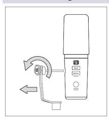
Revelator Dynamic can be removed from its yoke for comfortable handheld use or for mounting to a 1/4"-20 mic stand mount.
