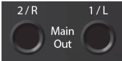
These are the Main outputs for the AudioBox GO. The output level of the Main outputs is controlled by the Main level control on the front of the unit. Playback streams 1 and 2 are routed to these outputs.
