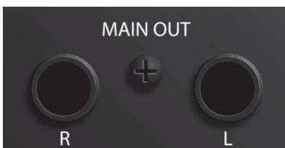
**Main Outs.** These are the Main outputs for the Revelator io44. The output level of the Main outputs is controlled by the Main level control on the front of the unit. Playback streams 1 and 2 are routed to these outputs.
