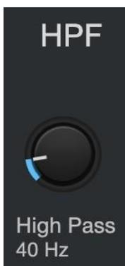
Use this control to set the High-Pass Filter frequency threshold for the selected Channel or Output Bus. The filter's threshold can be set from 24 Hz to 1 kHz. When the threshold is set to its lowest point, the filter is off. The high-pass filter's slope is -12 dB/8va.
