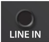
**Line In.** This 1/8-inch TRS input is suitable for line-level stereo sources like DJ mixers, mobile devices, synthesizers, and more.
