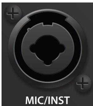
**Mic/Inst input.** Channel 1 of your Revelator io44 interface is equipped with a combo jack. This convenient connector accepts either a 1/4-inch TS connection for high-impedance instrument sources like guitars and basses, or an XLR connector for professional microphones. The XLR connection's XMAX-L solid-state microphone preamp is optimized for bus power.
