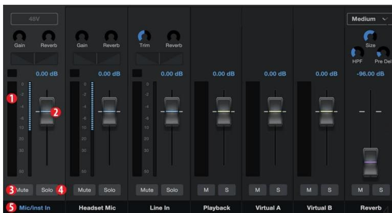
**Channel Meter.** This meter displays the current level of the channel before the fader (#2) level.
