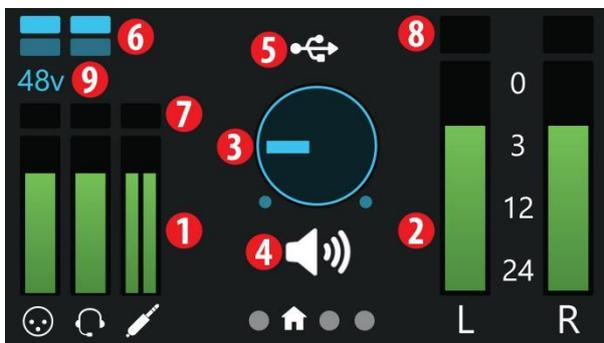
1. **Input Meters.** These meters indicate the input level of the analog inputs on your Revelator io44. The red Clip indicator will light when your input signal reaches -0.5 dBFS. At this level, the signal will begin to overload the analog-to-digital converters and exhibit signs of clipping. Use the gain controls to keep the signal below this level.
