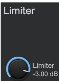
This encoder sets the threshold of the limiter for the selected channel or output bus. When the signal's amplitude (level) exceeds the threshold setting, the limiter is engaged. Turning the knob counterclockwise lowers the threshold, so limiting begins at a lower amplitude. The Limiter ratio is  $\infty:1$ .
