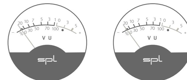
The ballistics of the VU meters guarantee an optimal visual perception. The time calibration of the VU meters complies with the requirements of the BBC. The rise time up to 0 dB is about 300 ms.
