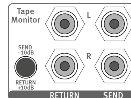
If no external device is connected set the TAPE MONITOR switch to Off. Otherwise the audio signal is interrupted.
