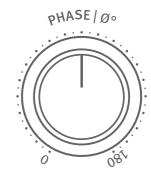
If you set the Phase switch to position "Var 0°", you set the phase of the LOW signal with the phase potentiometer from 0° to 180°.
