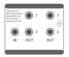
The Crossover has four trigger AMP CTL Outputs (20) to switch on up to four power amplifiers simultaneously. If the Crossover is triggered via its AMP CTL IN, the connected power amplifiers are triggered too.
