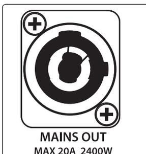
**Power Thru.** CDL-series loudspeakers provide loop-thru power. Using powerCON® Loop-thru cables and an AC powerCON Power cord, you can power up to six CDL-series loudspeakers on a single 15 amp / 120V (8 am / 240V electrical circuit).
