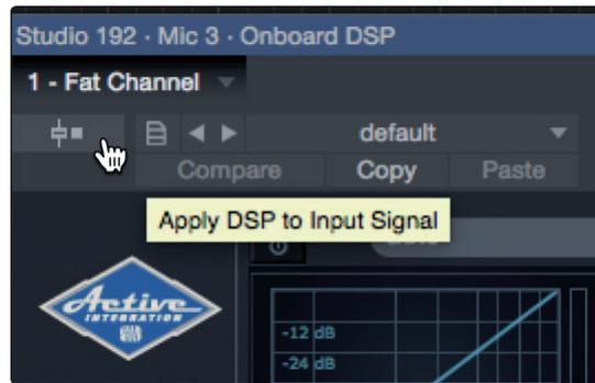
To listen your recordings through the same Fat Channel processing as the audio you are monitoring, simply drag the DSP Fat Channel plugin down to the channel insert to load an instance of the native Fat Channel plugin.
