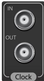
**Clock In and Out.** These BNC connections allow the Studio 192-series interface to receive and transmit word clock to and from other digital audio devices.
