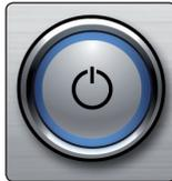
**Power button and Sync light.** The lighted ring around the power button of your Studio 192-series interface is a clock source / sync indicator. It lets you know if you unit is receiving word clock correctly.
