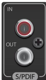
**S/PDIF In and Out.** The S/PDIF connections allow two channels of audio to be transmitted and received at rates up to 24-bit, 96 kHz. The S/PDIF I/O also allows the Studio 192-series interfaces to send and receive word clock to external digital devices.
