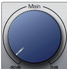
**Main.** The main knob controls the output level for the main outputs on the back of the Studio 192-series interface and has a range of -80 dB to 0 dB. This control provides attenuation only.
