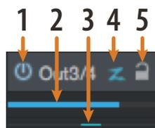
1. **Activate Button.** To completely remove any channel from a Z-Mix, simply deactivate the Z-Mix object for that channel. In most instances, you will leave this enabled.
