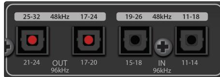
**ADAT – S/MUX In and Out.** These are the ADAT – Dual S/MUX connections for your external digital devices. When recording or playing back at 44.1 or 48 kHz, each ADAT I/O will provide 8 of the 16 available channels consecutively, from left to right. When recording or playing back at 88.2 or 96 kHz, each connection will provide four of the available eight channels.
