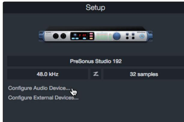
**Power User Tip:** If your device has zero-latency monitoring functionality from within Studio One, you will see the Z-mix icon. If you do not see this icon, make sure that you have launched Universal Control or Universal Control-AI. PreSonus audio interfaces require their DSP mixing control panels to be running in the background for Z-mix functionality.
