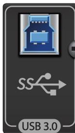
**USB 3.0 port.** Use this port to connect your Studio 192-series interface to your computer. While the Studio 192-series interface is a true USB 3.0 device, it is fully backwards compatible with USB 2.0 connections. Do not connect your Studio 192-series interface to a USB 1.1 or lower connection on your computer.
