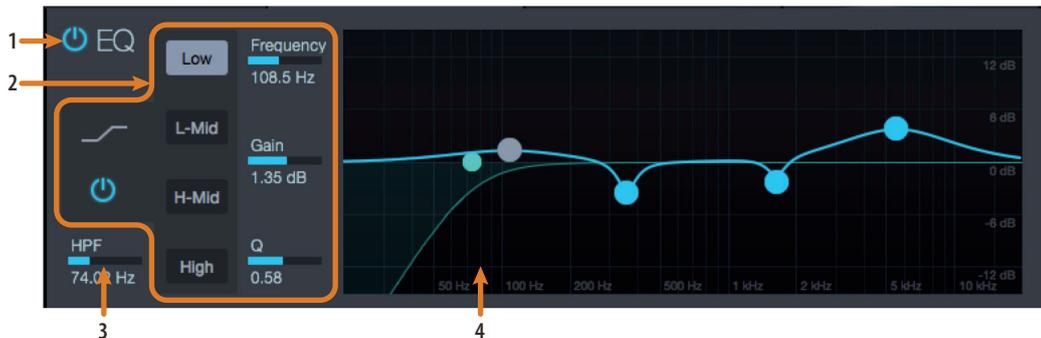
1. **Equalizer On/Off.** Turns EQ on or off for the selected analog input channel.
