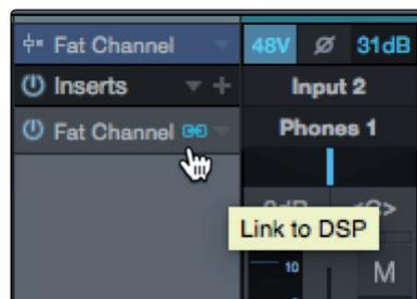
**Power User Tip:** You can also drag in your favorite Fat Channel plugin presets from the Browser. Once inserted on your channel, clicking the “link to DSP” button will copy that preset to your DSP Fat Channel. This bidirectional workflow allows you to copy settings from your DSP Fat Channel to your DAW insert or vice versa.
