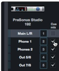
**Power User Tip:** It is possible to designate the main output as a cue mix. This is helpful if you often record yourself and require quick access to zero-latency monitoring for live inputs. When the main output is designated as a Z-Mix, a Zero Latency button will appear on any audio channel, with an assigned audio input in the Console, below the Mute, Solo, Record, and Monitor buttons.
