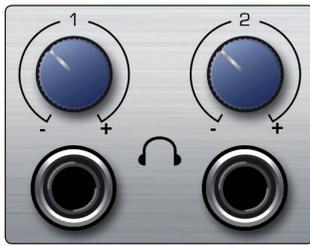
**Headphones Outputs.** Your Studio 192-series interface provides two/one headphone outputs, each with its own level control. Each headphone output is provided with its own unique output stream to route audio directly from your DAW (Studio 192: playback streams 11-12 and 13-14, Studio 192 Mobile: playback streams 7-8). From UC Surface, any mix can be routed to either headphone output.
