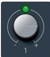
**Input Gain Controls.** These knobs provide 80 dB of variable gain for Mic and Instrument; 40 dB of range for Line (-20 to +20)
