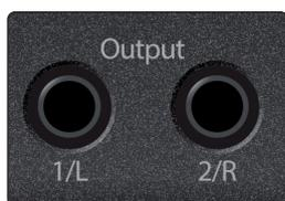
**Main Outs.** These are the Main outputs for the ioStation 24c. The output level of the Main outputs is controlled by the Main level control on the front of the unit. Playback streams 1 and 2 are routed to these outputs.
