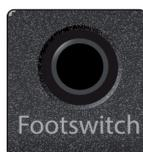
**Footswitch.** Use this port to connect a footswitch to your ioStation 24c to trigger start/stop or recording punch-ins. The ioStation 24c will auto-detect the footswitch polarity upon power-up and conform to the footswitch that is connected to it. Either a momentary or a latching switch can be used.
