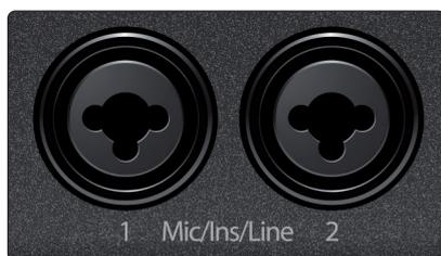
**Mic/Ins/Line inputs** Your ioStation 24c interface is equipped with high-quality XMAX microphone preamplifiers for use with all types of microphones.
