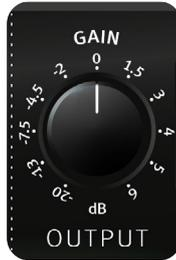
The outgoing signal can either be dampened to -20 dB or further amplified by +6 dB with the Output control to provide optimal drive to the subsequent units or the optional AD converter. The selected output level is shown on the PPM OUTPUT display in the display field.
