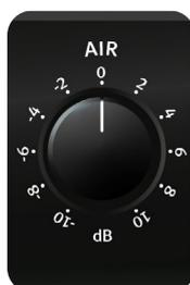
The high frequency filter in the equalizer module is described as AIR. A coil-capacitor filter with so called bell characteristics and a center frequency of 19 kHz comes into operation here. At this frequency the maximum possible accentuation is +10 dB, the maximum possible damping is -10 dB.
