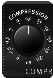
The Compression control can be used to set a threshold between 0 dB and -20 dB. The lower the threshold, the more the compressor works.
