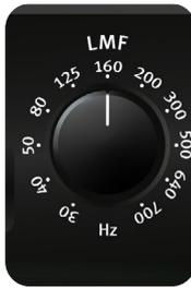
The center frequency of the half-parametric low/mid frequency filter is set with the LMF control (low/mid frequencies). The adjustable frequency range is between 30 Hz and 700 Hz so that this filter covers a range of about 4.5 octaves, allowing it to be used from the deepest bass to the lower mid range. This together with the MHF filter ensures that the entire frequency spectrum is covered.
