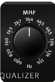
The center frequency of the semi-parametric mid/high frequency filter is set with the MHF control. (MHF: mid/high frequencies). The frequency range can be set between 680 Hz and 15 kHz so that this filter covers a range of 4.5 octaves and can be equally be used in the lower mid as well as the high frequency.
