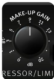
The Make-Up Gain control can be used to make up for the overall level reduction caused by compression. A value between 0 dB and 20 dB can be set by which the level is increased again after compression.
