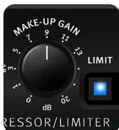
The Limiter switch puts the compressor into limiter mode. The threshold is still set by the compression knob.
