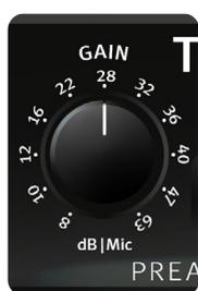
The gain control can be used to adjust the preamplification. For microphone signals, a preamplification of up to 63 dB can be realized. When optionally equipped with an input transformer, approximately +14 dB must be added to the scaled values.
