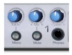
• ExtIn. The external in knob controls the input level and amount of the Stereo Ext. In on the rear of the chassis for the channel.
