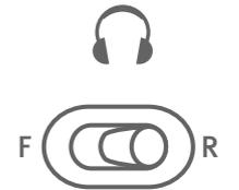
Set to the R setting, the headphone signal passes through to both the headhone connectors on the rear side.
