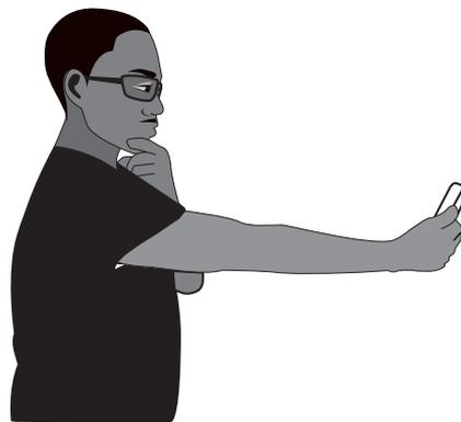
The SPL meter should be held at arm’s length, with the microphone pointed at the center point between the left and right speakers (where your head will be), angled at 45 degrees to ensure an accurate reading. If your SPL meter is also your cell phone, make sure your finger or cell phone case isn’t covering the mic!
