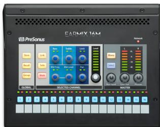
**EarMix 16M Personal Monitor Mixer.** The PreSonus EarMix 16M personal monitor mixer provides 16 input channels over AVB each with 3-band EQ and limiter. Power-over-Ethernet (PoE) allows for easy deployment.
