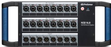
**NSB-series stage boxes.** The NSB 8.8 and NSB 16.8 offers 8 or 16 locking combo mic/line inputs with remote-controlled XMAX preamps that include gain compensation for shared input scenarios. Eight outputs employ locking XLR jacks. A built-in 2-port AVB switch lets you daisy-chain multiple units.
