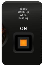
The On switch is used to activate the Vitalizer Mk3-T.
