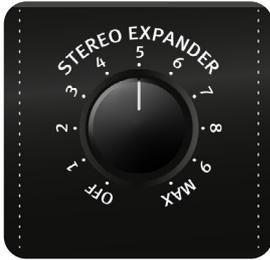
The Stereo Expander increases the width of the stereo image.
