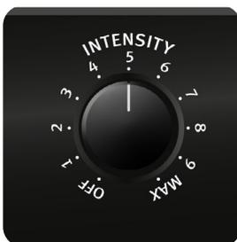
The Intensity control determines the level of the LC-EQ. As the intensity increases, the gain of the set high and mid-hi frequencies increases. At the same time, the perception time is shifted so that soft high-frequency components are not masked by loud ones. This improves speech intelligibility and clarity. The brilliance of any audio signal can be increased without sounding sharp.
