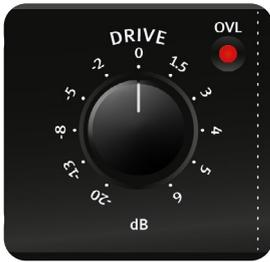
Drive controls the level going into the filter network. The control range of the level is between -20 dB and +6 dB. In the center position (0dB) the drive level is identical to the input level.
